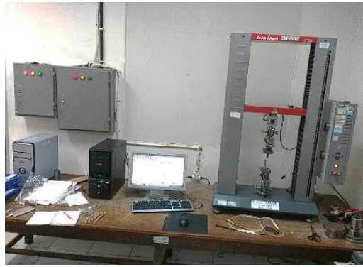
Figure 4. Zwick Roell Z020 Tensile Testing Setup
