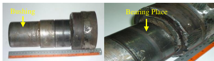
Figure 3. The fracture shaft is between Ø65 mm to Ø90 mm.
