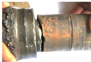
Figure 1. The fracture shaft of oil palm lorry S45C 2,640 working hours.
