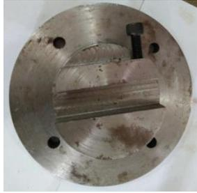
**Gambar 7.** Memasang *toolpost lower* terhadap *upper tool*
