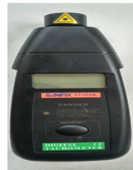
Gambar 2. Alat ukur putaran mesin ( Tachometer )
