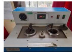
**Gambar 7.** Viskometer
