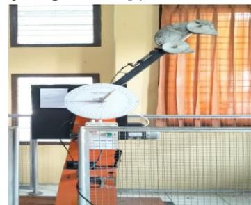
**Gambar 1.** Alat Uji Impak *Charpy*
