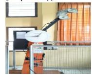
Gambar 1. Alat Uji Impak Charpy
