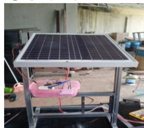
**Gambar 1.** Panel Surya tipe *poly-crystalline*
