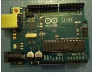
Gambar 2. Microcontroller Arduino Uno
